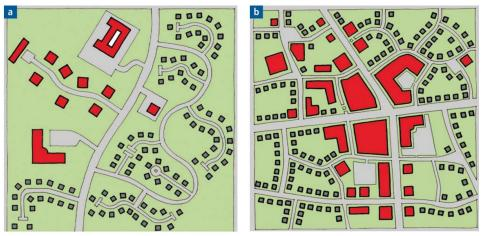
**Figure 6: Route connectivity** – In typical post-WW2 developments (a) the main roads are often the only through routes. In more historic areas (b) there may be parallel routes that could be made suitable for cycling (<u>Manual for Streets</u> and <u>LTN 1/20</u>, Department for Transport)
