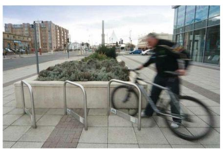
**Figure 7: Sheffield stands** – setting with natural surveillance, accessible and integrated into street furniture
