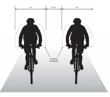
**Figure 4: Dynamic kinetic envelope of cyclists** (<u>LTN 1/20: Cycle Infrastructure Design</u>, Department for Transport)
