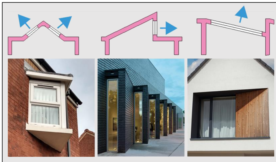
Figure 4.10: Maintaining privacy by varying window orientation
