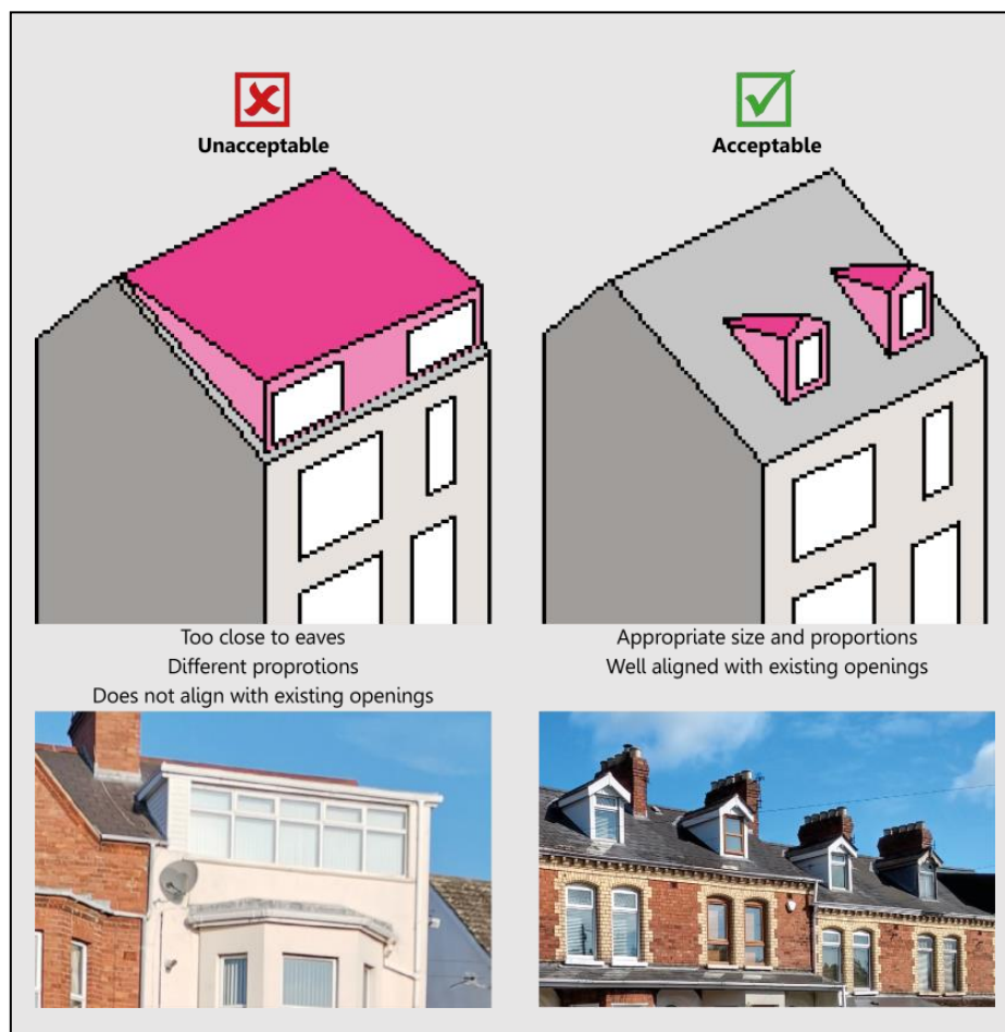
Figure 4.6: Roof extensions and dormers
